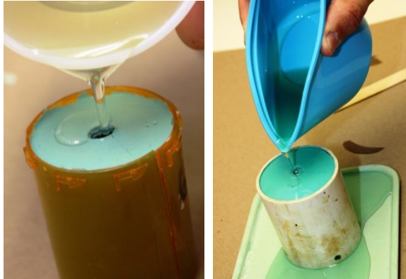
Figure 12. Pouring the molding resin into the mold through the hole in the mold.
