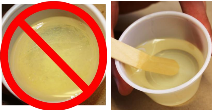
Figure 10. Two-part resin compound not fully mixed.
