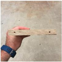
Insert screw eyes in pilot holes (#12 for plastic back, #10 for wooden back)
