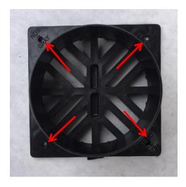
Lay the basket top down and center the drain cover on the bottom of the basket with the grate against the wire. Secure in place with one zip tie in each corner and one in middle running perpendicular to the zip ties in the corners (this will prevent the basket from sliding). Trim zip ties.
