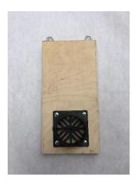
For the plastic back, drill four holes in back board to line up with holes in grate and secure in place with machine screws (screw heads on back of board, washers & nuts on front [drain] side)
